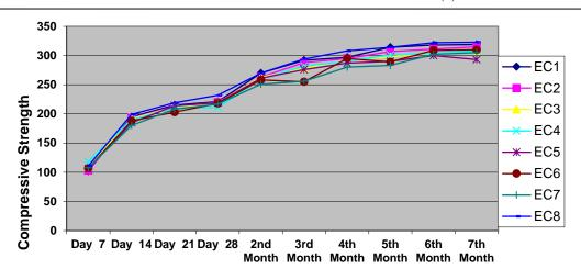
Figure 9: Compressive strength of the samples at different periods of time.
