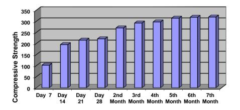
Figure 1: Compressive strengths of samples placed in water with EC from 0 to 3000.
