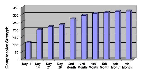
Figure 8: Compressive strengths of samples placed in water with EC of max 300.
