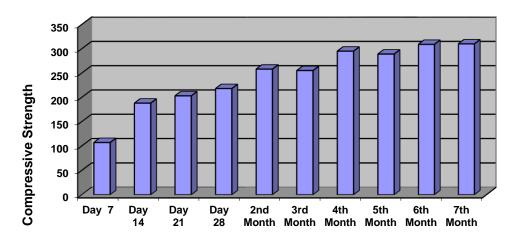
Figure 6: Compressive strengths of samples placed in water with EC from 15000 to 18000.
