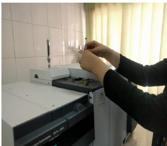
Figure 2: Gas chromatography/mass spectrometer (right side) and how to inject into it (left side).
