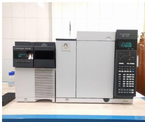
Figure 2: Gas chromatography/mass spectrometer (right side) and how to inject into it (left side).
