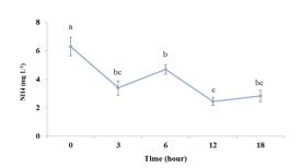
Figure 7: The variation of  $\mathrm{NH_4}^+$  changes in the nanoparticle reactor during the study period.
