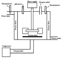
Figure 4: A complete schematic of the designed reactor.
