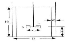
Figure 1: standards of reservoir reactor dimensions (Katoh and Yoshida, 2009)
