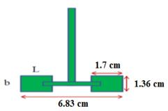
Figure 2: Schematic of the designed mixer.
