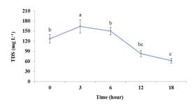
Figure6: The variation of TDS changes in the nanoparticle reactor during the study period.
