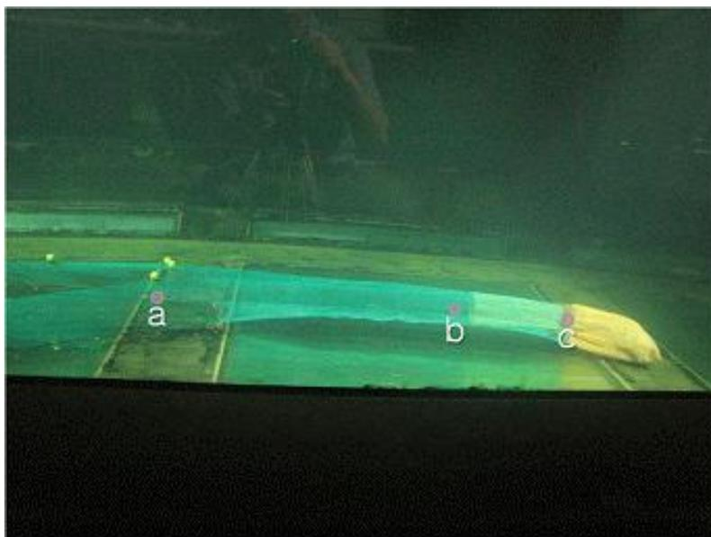
Figure 4: Measuring the change in speed of the water flow in the model fishing gear. If the flow speed is reduced due to the BRD, then shrimp could escape
