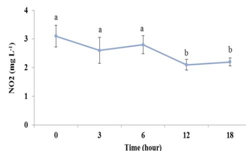
**Figure 11 :** The variation of NO<sub>2</sub><sup>-</sup> changes in the nanoparticle reactor during the study period.
