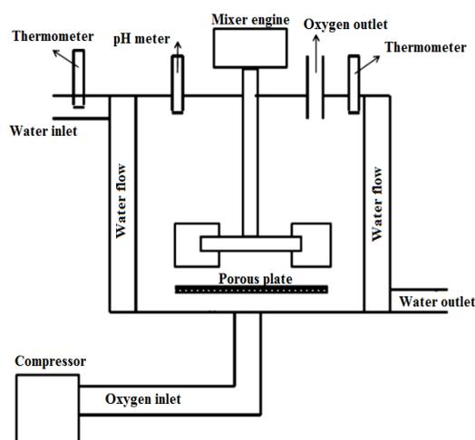
Figure 4: A complete schematic of the designed reactor.
