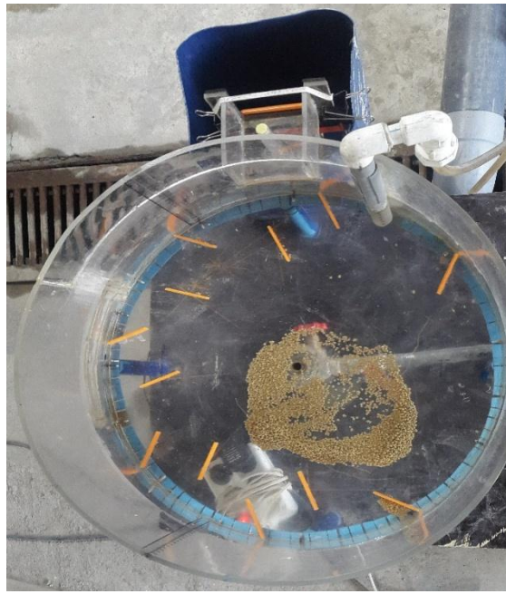
Figure 4: Sample of sedimentation in cylindrical tank.
