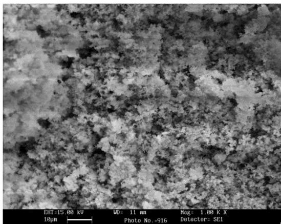
**Figure3:Electron-microscopic images of non-molecularly imprinted polymer (NIP)-magnification 5.00 KX, with particle diameter 2 µm.**
