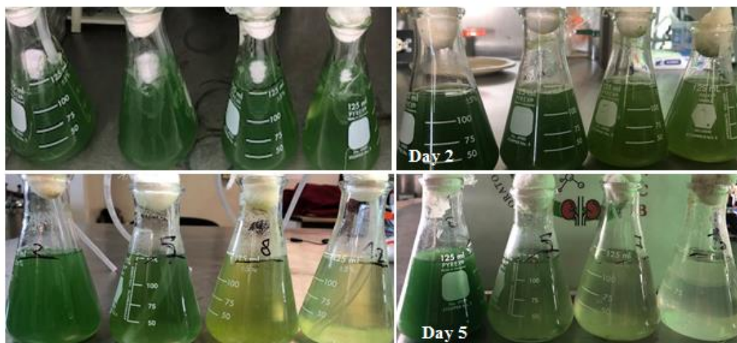
Figure 3: Changes in medium's color during cultivation day (from right to left show four different concentrations of ammonium sulfate of 0, 1.25, 2.5 and 5 gL -1 , respectively)
