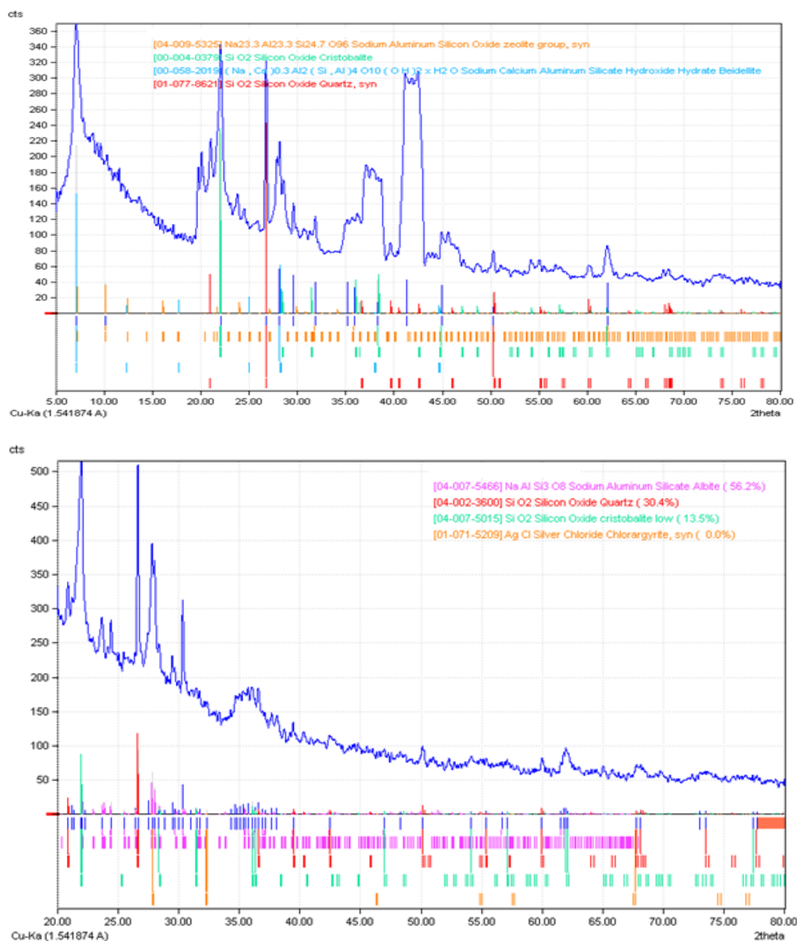
Figure 6: XRD analysis of raw bentonite (above) and silver nanoparticle-coated (below) bentonite.
