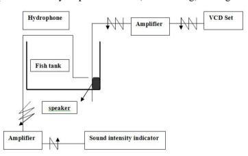
Figure 1: Schematic diagram of music transmission in goldfish tank and hydrophone output recording.
