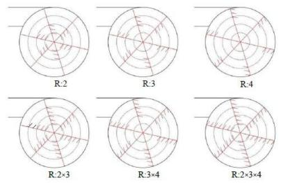
Figure 2: Six different arrangements of vane on the bed of settling basin.
