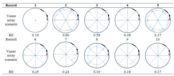
Figure 4: sediments discharge efficiency of different scenarios for application of submerged vanes in different arrays.
