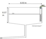
Figure 3: Typical scheme of laboratory 'Cornell-type' dual-drain tank.
