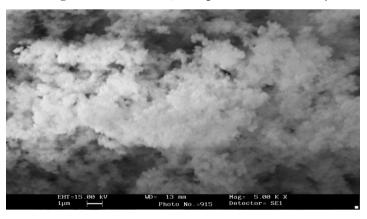
Figure 2: Molecularly imprinted polymer (MIP)- magnification 5.00 KX, with particle diameter 1  $\mu m.$
