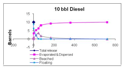
Figure 5: Diesel degradation chart, 10 bbl
