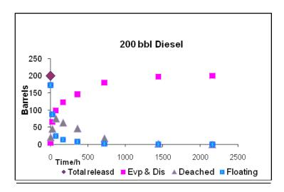
Figure 6: diesel degradation chart, 200 bbl
