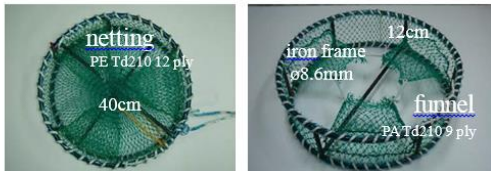
Figure 2: The net pot used for catching the common octopus in the coastal sea of Korea.
